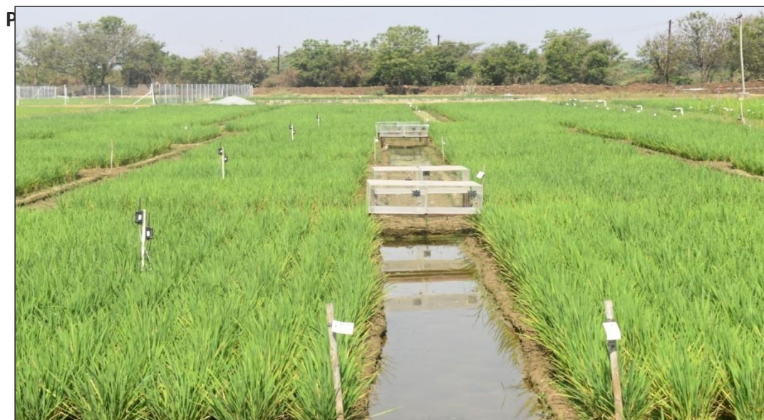
Plate . IoT water meters, water level Sensors installed in the experimental field.
